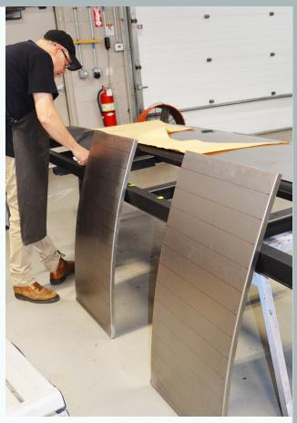
All panels on the bus body are being replaced with new panels. This is due to to all of the damage incurred over the years. The panels above are for the rear of the bus body. Sam has made them and with the Pullmax machine has duplicated the bead on the bottom of the panel
