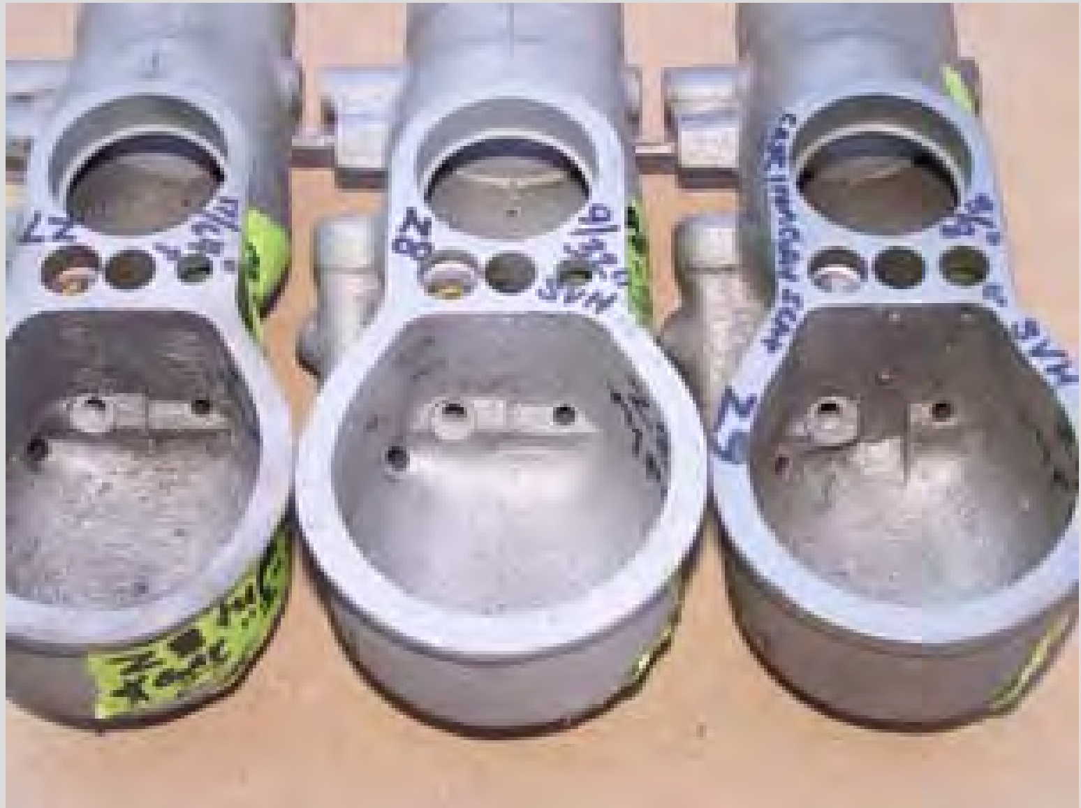
Fig. 17: The Mid 1929 Z7, Late 1929 Z8, & 1930 Z9 SVH difference and comparison.
