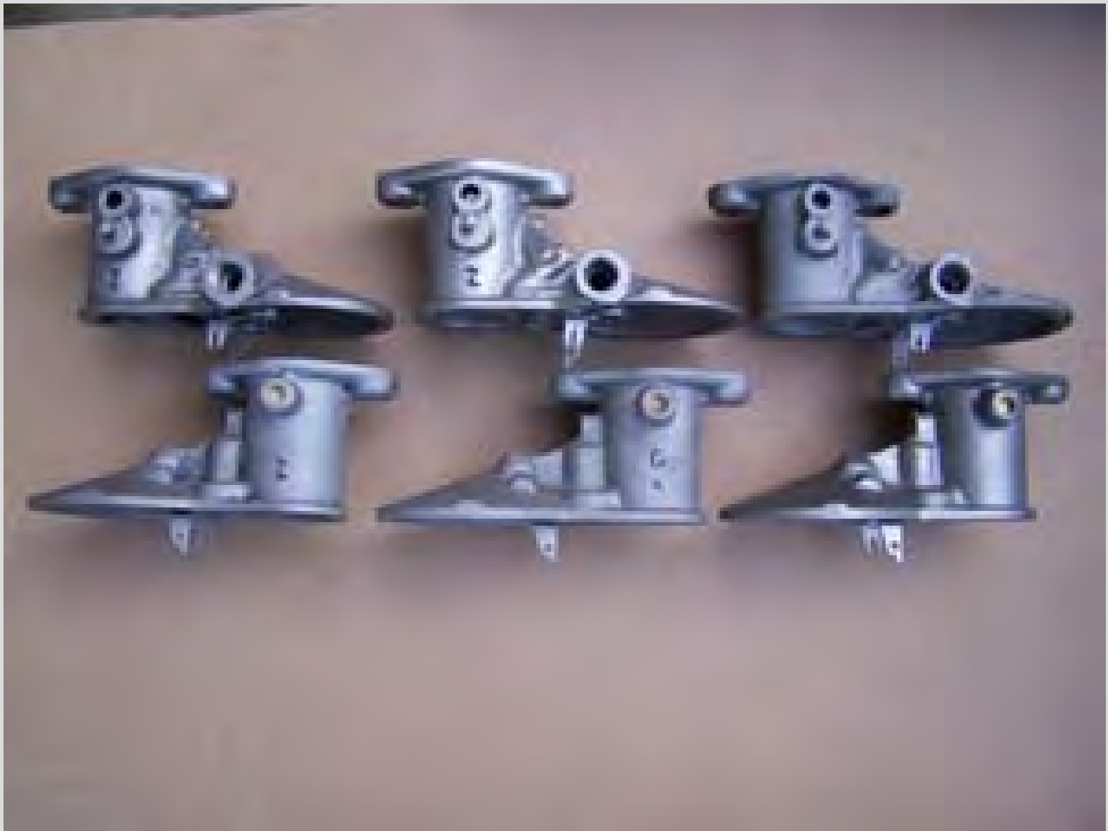
Fig. 22: The 1931 Z13, Z14, & Z15 side bowl carburetor top castings. Front & backside views.
