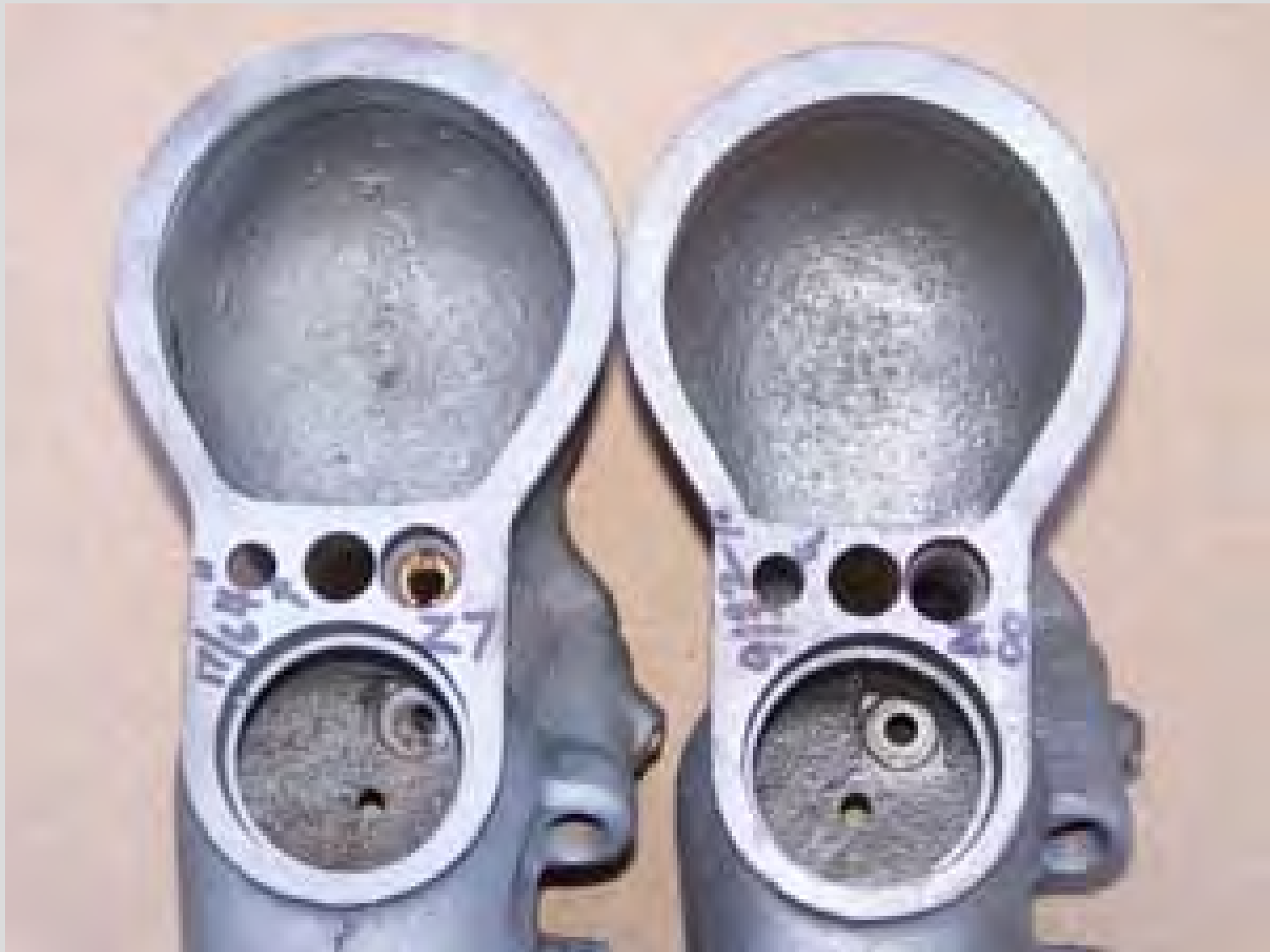
Fig. 12: The Mid 1929 Z7 & Late 1929 Z8 carburetor SVH difference.
