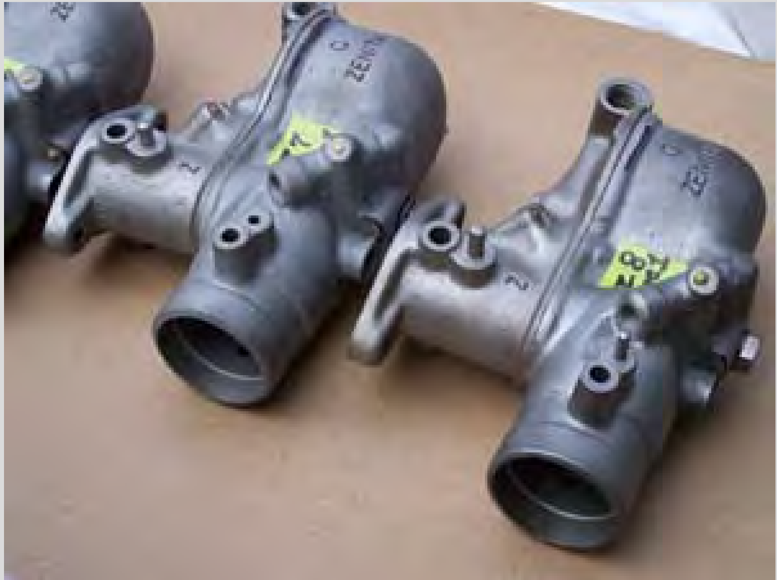
Fig. 8: The 1929 Z6, Z7, & Z8 carburetors. Oblique view of the “area below the GAV boss.”
