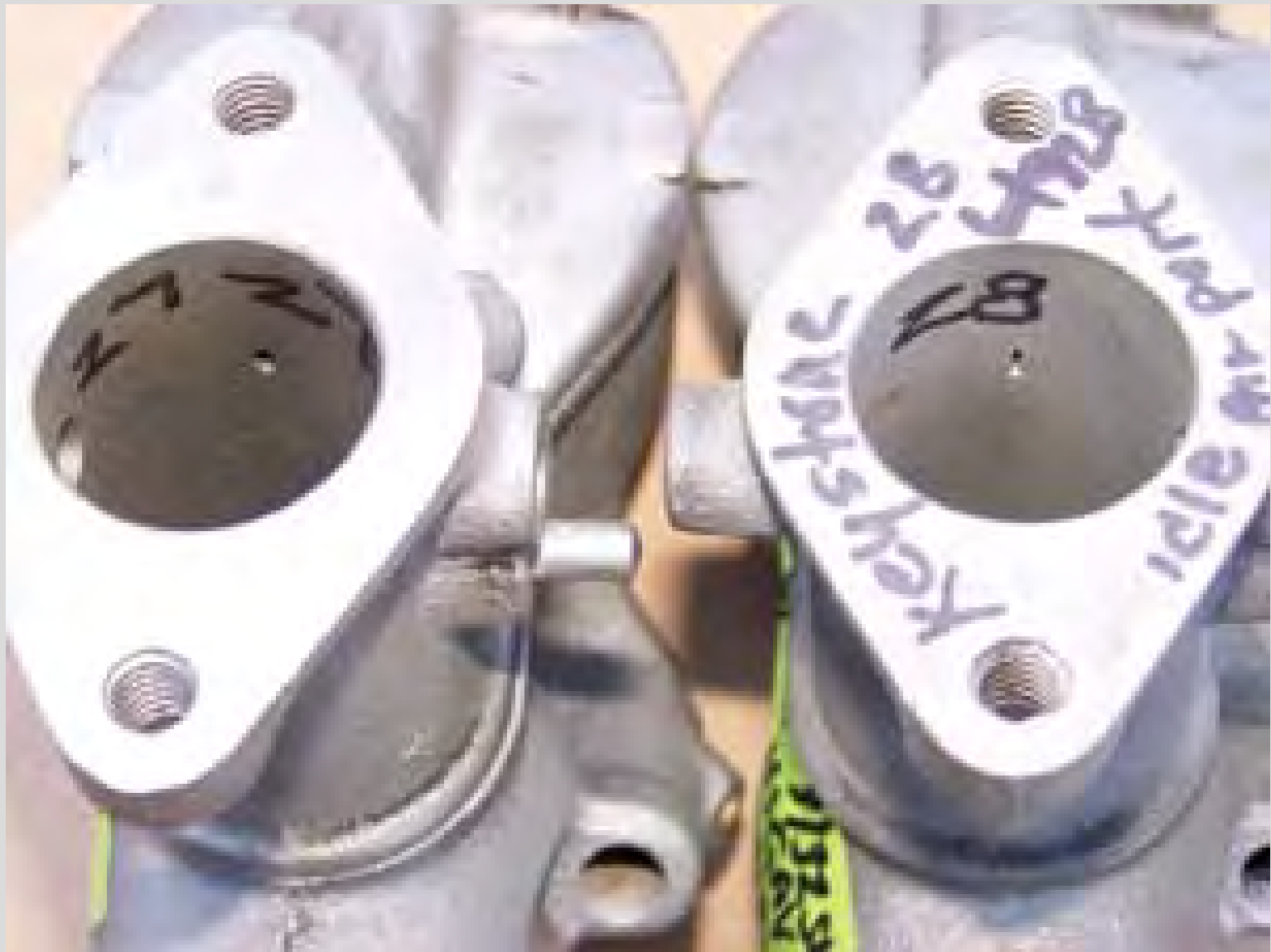
Fig. 13: The Mid 1929 Z7 & Late 1929 Z8 carburetor "Idle Air Passage" differences.
