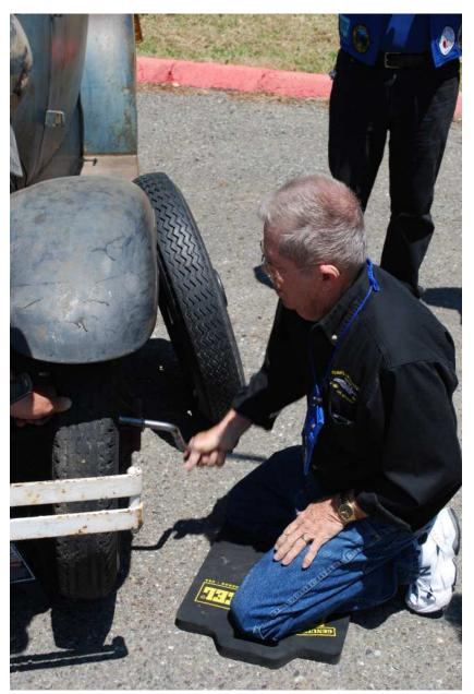
NOTE: Once all contestants are done, ensure lug nuts are properly tightened before vehicle drives off – 64 ft. lbs. is recommended.
