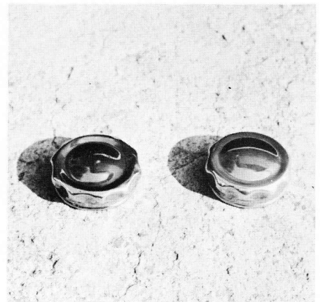
EARLY RADIATOR CAP at left has deeper recess around top than later model at right.
