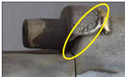
Cut slot window area (circled) with stress crack below
