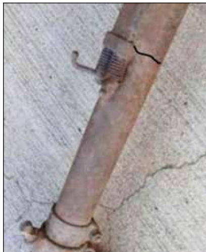
Cut slot window area (circled) with stress crack below
