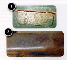
Assuming you've determined the original engine or frame number, the vehicle assembly date could be as much as 3 months after the engine production date (4 months in 1931) and 6 months for commercial vehicles.
