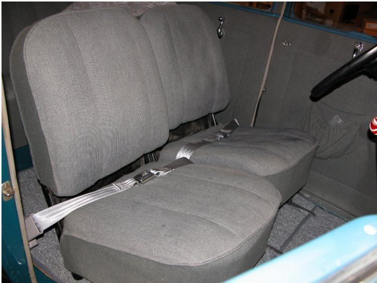
Once you have the seats back in, have someone sit in each set and adjust the angle of the retractors so that the belt pulls straight out of the unit, then tighten their attachment bolts.
